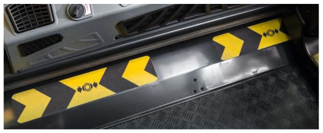
Conventional pedals are no longer included, increasing both the viewing scope for the driver and the movability of his seat.
